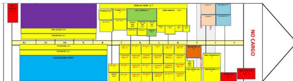
Figure 6: Loading condition of Anahita. The purple-coloured box indicates the area occupied by casing joints before the occurrence. (Source: Company. Annotated by TSIB)
